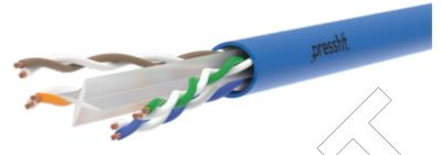
Pressfit CAT 6 LAN cables are manufactured using solid, bright annealed copper conductor, insulated with a high-density polyethylene compound. These offer low attenuation, low cross talk, and low return loss. They are also commonly referred to as Ethernet cables or simply, CAT cables.
