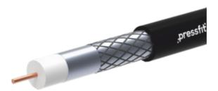
RG-6 Coaxial cables are single-core electrical wires with a solid annealed copper core that is insulated with polyethylene and shielded with a metal foil. They are further encased with fine aluminum mesh to provide the necessary shielding against noise. Lastly, this entire structure is further insulated to keep it intact and protect it from abrasion and disruptions.
