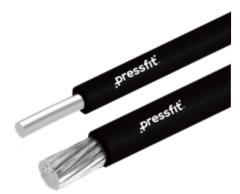
Pressfit's Alu-Line single core building wires are manufactured using bright electrolytic grade aluminium, delivering 64% conductivity. The wires are drawn and annealed into a circular conductor which has consistent resistance and is also compact. The insulation of the wires is made from a special grade of UV-resistant PVC compound and can withstand harsh weather conditions, providing higher electrical safety.
